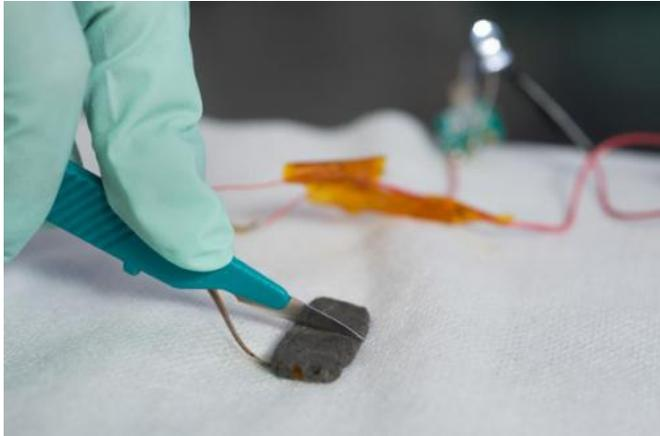
A small piece of the self-healing material is sliced with a scalpel. The researchers say the material repairs itself in about 30 minutes. Credit: L.A. Cicero
