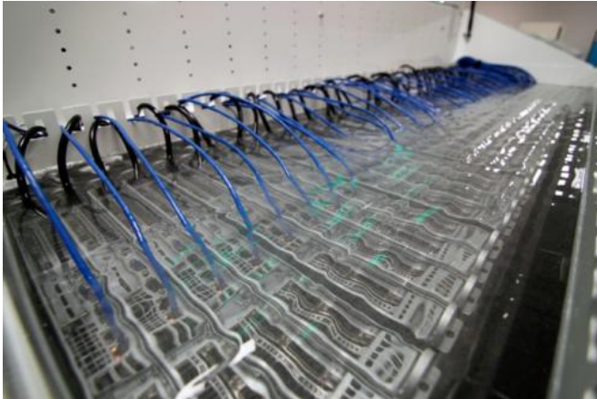
Supermicro SuperServers submerged at CGGVeritas
