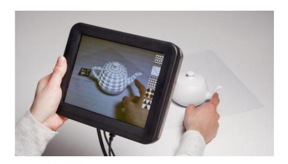
REVEL is a new wearable tactile technology that modifies the user's tactile perception of the physical world. As a result, it can provide a layer of artificial tactile texture on almost any surface or object, including touch-screens, walls, furniture, plastic or wooden objects, and even human skin. Revel requires little, if any, instrumentation of the physical world.
