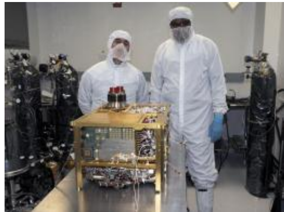
The Sample Analysis at Mars (SAM) instrument for NASA's Mars Science Laboratory mission will study chemistry of rocks, soil and air as the mission's rover, Curiosity, investigates Gale Crater on Mars. SAM was built at the NASA Goddard Space Flight Center, Greenbelt, Md., where this image was taken. Image credit: NASA
