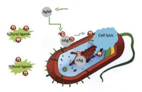
Silver ions delivered by nanoparticles to bacteria promote lysis, the process by which cells break down and ultimately die, which makes silver nanoparticles a superior and widely used antibacterial agent. New research by Rice University found that silver ions, not the particles themselves, are toxic to bacteria. They also found that ligands in the vicinity of a bacteria can bind silver ions and prevent them from reaching their target. Credit: Zongming Xiu/Rice University
