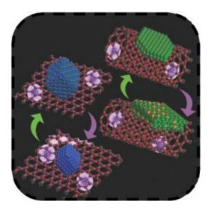
The nanocrystal structures used in the batteries. Green arrows represent discharging, while purple represent charging. Current flows in through the iron-carbon nanostructure (left) and out through the nickel-carbon nanotube structure (right).
