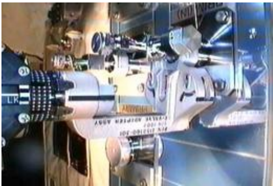
RRM's Multifunction Tool with its T-Valve Adapter closes in to retrieve the T-Valve on the RRM module. Credit: NASA
