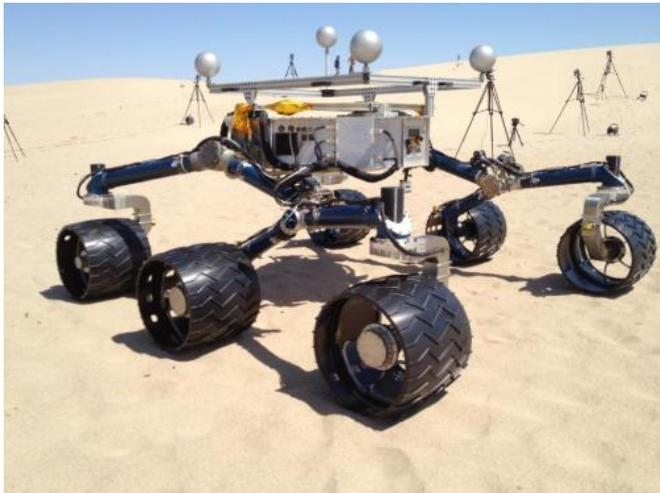
Mars Science Laboratory mission team members ran mobility tests on California sand dunes in early May 2012 in preparation for operating the Curiosity rover, currently en route to Mars, after its landing in Mars' Gale Crater. Credit: NASA/JPL-Caltech
