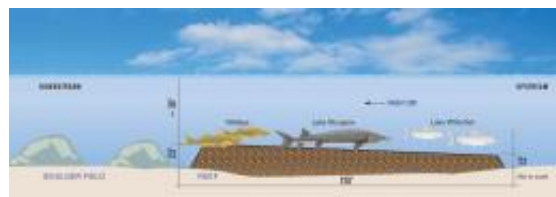
An illustration showing the dimensions of the rock reefs under construction on the St. Clair River. Credit: Michigan Sea Grant
