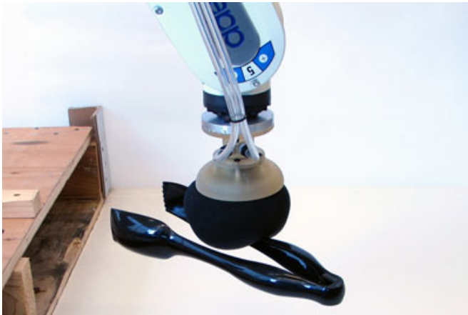
The universal jamming gripper picking up a pair of tongs. The trick is to decide where to grab.
