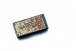
Imec's low-power 7Gbps 60GHz transceiver IC implemented in 40nm low-power CMOS.
