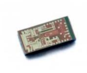
Imec's low-power 7Gbps 60GHz transceiver IC implemented in 40nm low-power CMOS.
