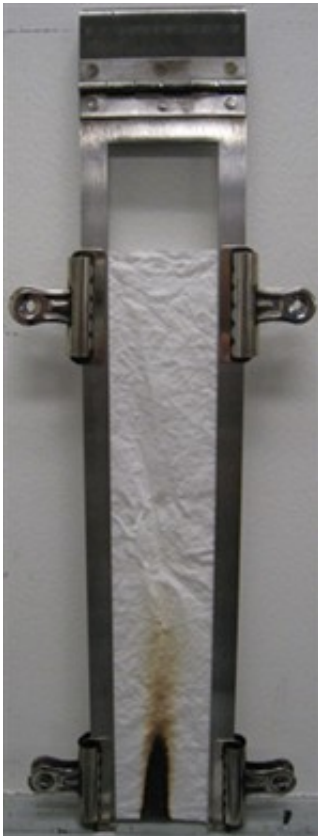
Cotton fabric after a vertical flame test, where a flame touches the fabric for 12 seconds
