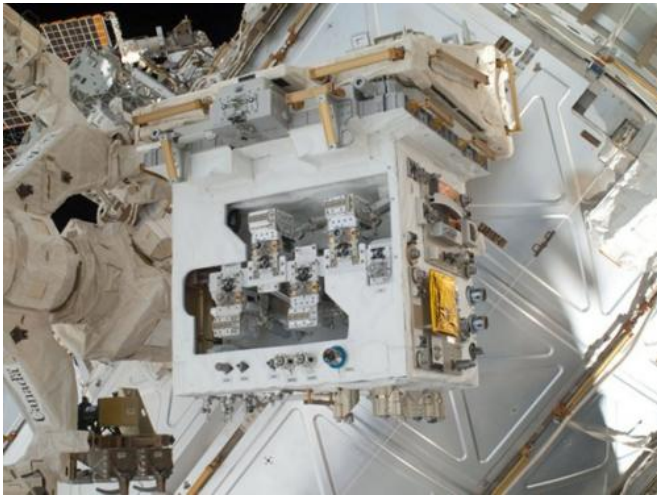
The Robotic Refueling Mission (RRM) module on the International Space Station before it was installed on its permanent platform. RRM will demonstrate robotic servicing technology and lay the foundation for future missions. Credit: NASA
