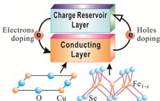
A view of structural unit of high-temperature cuprate- and iron selenide-based superconductors courtesy of Xiao-Jia Chen.
