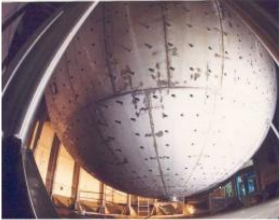
View of the Borexino "Stainless Steel Sphere" (SSS) from from the "Water Tank"
