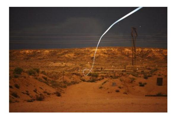
A tiny light-emitting diode, or LED, attached to a self-guided bullet at Sandia National Laboratories shows a bright path during a nighttime field test that proved the battery and electronics could survive the bullet's launch. (Photo courtesy of Sandia National Laboratories)
