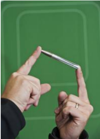
The four-inch-long bullet has actuators that steer tiny fins that guide it to its target. (Photo by Randy Montoya)
