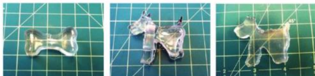
(A) A silicone sample started off in the shape of a dog bone. (B) The sample was cut into pieces and rearranged in a dog mold. (C) The sample was remolded into a dog, in which the fracture locations are undetectable. Image credit: Zheng, et al. ©2012 American Chemical Society
