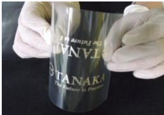
An electronic circuit created through flexographic printing using the silver ink. Image: Tanaka Kikinzoku Kogyo K.K.
