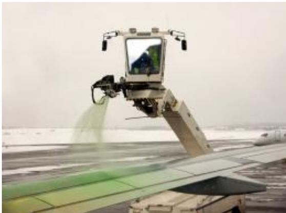
An aircraft wing being de-iced to avoid jeopardising air safety. (Photo: istockphoto)
