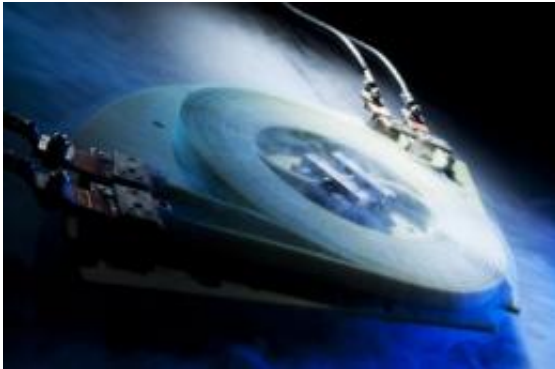
Superconducting coils are cooled with liquid nitrogen and have zero resistance to current flow. Credit: Martin Lober, KIT
