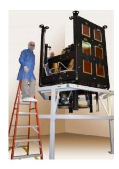
The Center Of Curvature Optical Assembly (COCOA) will allow the program to verify the optical performance of the 21.3-foot (6.5-meter) primary mirror at its 40 degrees Kelvin (-233 Celsius) operating temperature. The COCOA contains mechanical and optical instruments that allow the test team to identify, align and test the 18-segments from outside the vacuum chamber. Credit: Note: The background of this image has been digitally removed. Credit: ITT Exelis
