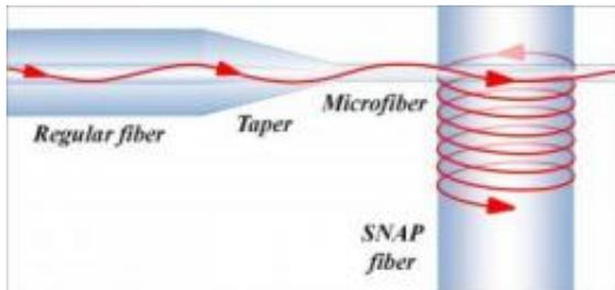
This figure shows the propagation of light in a SNAP fiber coupled to a tapered regular optical fiber. Credit: Courtesy OFS Laboratories
