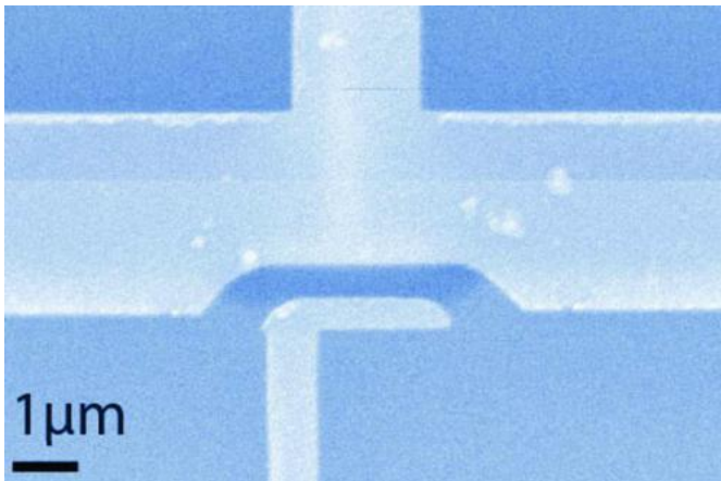
The suitcase-like handle are the two nanowires, one above the other. The darkest areas are gallium arsenide crystal. The two lighter areas in the shape of "plus" signs are gold gates at the top and bottom of the device. (Sandia scanning electron microscope image)
