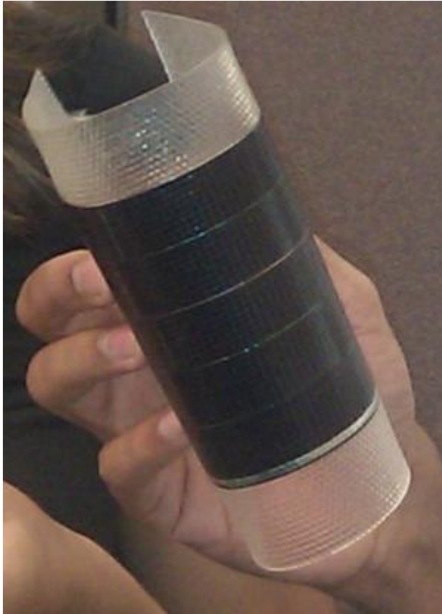
Thin film solar cells fabricated from gallium arsenide have achieved a record sunlight-to-electricity conversion efficiency of 28.4 percent. (Image courtesy of Alta Devices, Inc.)
