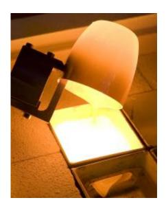
A robot arm takes over the fully automatic handling of the test melts in the glass screening unit - here, the pouring of the melt into the sample form. Credit: Knud Dobberke for Fraunhofer ISC
