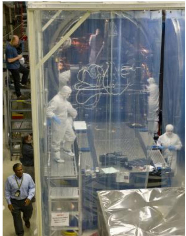
The TIRS instrument sits half out of the thermal vacuum chamber while still protected in a clean tent, as team members disconnect the electrical wires and cooling lines after testing. Credit:NASA/Goddard/Bill Hrybyk
