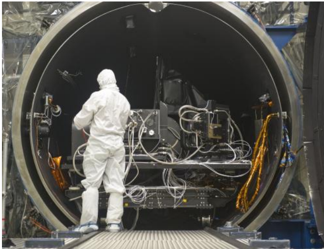
A technician surveys the TIRS instrument and the calibration equipment, preparing to move to the clean room after testing. Credit:NASA/Goddard/Bill Hrybyk
