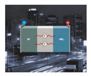
A fluoride-containing electrolyte separates the metal anode from the metal fluoride cathode. Credit: Figure: KIT
