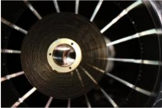
Each of the seven telescope modules consists of 54 nested special mirrors. Image: MPE
