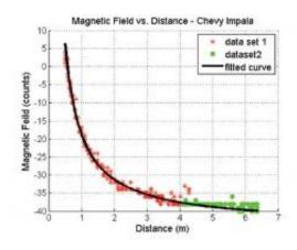
By determining a clear inverse relationship between a vehicle's magnetic field and its distance (obtained from a sonar sensor), scientists can estimate the distance between two vehicles at close spacing with a simple, inexpensive sensor. Image credit: S. Taghvaeeyan and R. Rajamani. ©2011 American Institute of Physics
