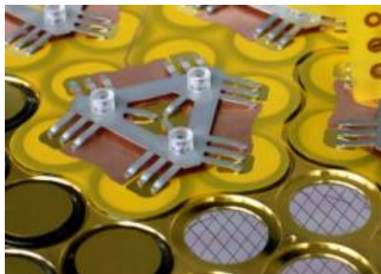
A collection of seven avalanche photodiodes, the sensors that detect instances of two-neutrino double-beta decay (as well as other decays), makes a spider, as shown at right. More than 40 spiders make up a detector. Credit: EXO Collaboration.
