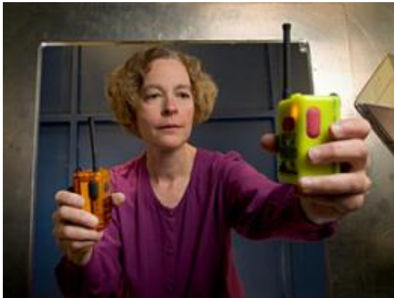
NIST engineer Kate Remley holds two Personal Alert Safety System (PASS) devices with wireless alarm capability. Credit: Paul Trantow/Altitude Arts
