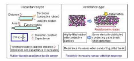
This table displays the capacitance and resistance-type Smart Rubber sensors in RIBA-II. Credit: RIKEN
