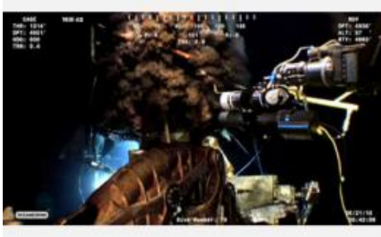
The manipulator arm of a robotic vehicle (upper right) moves a sampler toward hot oil and gas. Credit: Oceaneering
