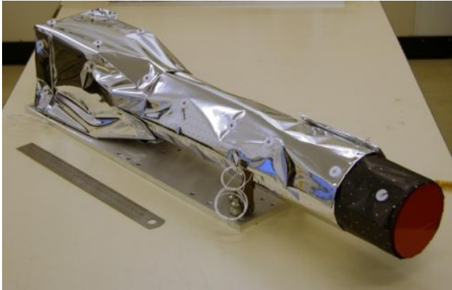
The flight model of the medium resolution camera, RAL Cam 3, to be installed on the International Space Station
