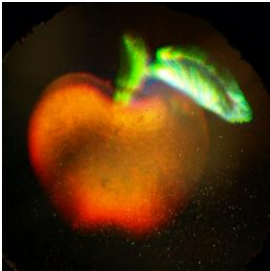
Figure 1: A full-color holographic apple achieved using surface plasmon polaritons in a silver film. Reproduced, with permission from, Ref. 1 © 2011 AAAS
