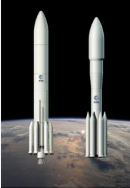
NGL concepts under study - Left: main stage powered by a cryogenic liquid oxygen and hydrogen engine (staged combustion cycle), with a cryogenic reignitable engine for the upper stage. Right: first two stages powered by solid propellants, with a cryogenic reignitable engine for the upper stage. Credits: ESA - D. Ducros
