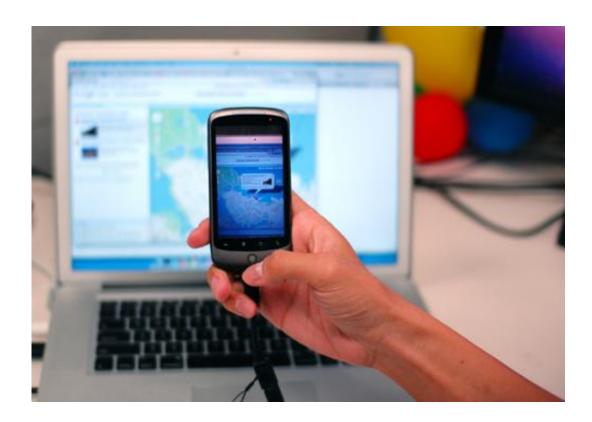
When Deep Shot transfers an open application to a cellphone, it automatically resizes the application window to match the framing of the photo. *Photo courtesy of Tsung-Hsiang Chang*
