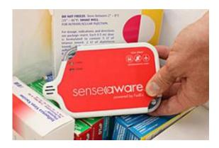
Developed by international shipper FedEx and tested with help from NIST, the Senseaware device connects to cell phone networks to provide users with near real-time information on a package's precise location, temperature, humidity, pressure, acceleration, elevation and exposure to light. NIST researchers plan to deploy the technology as part of a pilot project to monitor and improve climate measurements. Credit: Strouse/NIST
