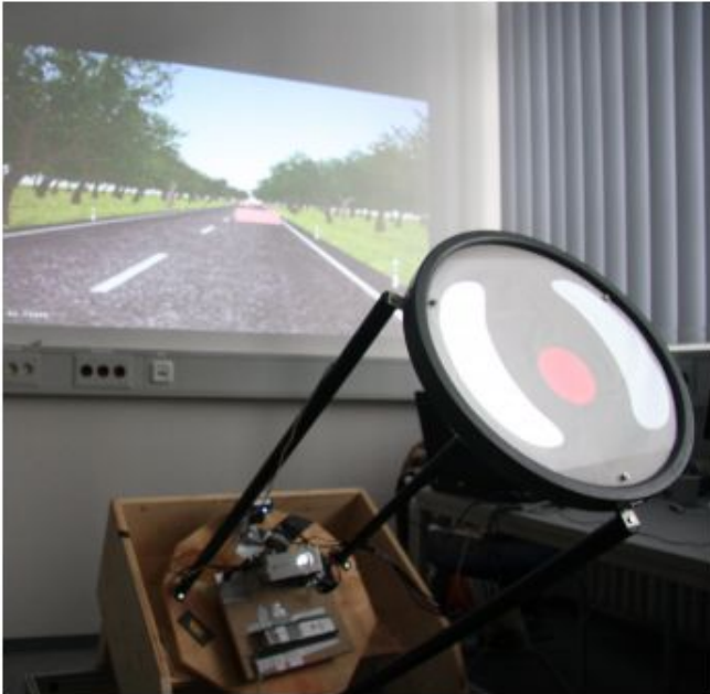
The multi-touch steering wheel hardware. Image: Tanja Döring et al.
