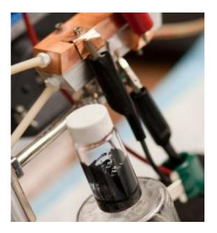
A sample of 'Cambridge crude' — a black, gooey substance that can power a highly efficient new type of battery. A prototype of the semi-solid flow battery is seen behind the flask. Photo: Dominick Reuter
