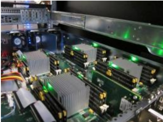
This is a view of the internals of the Moneta storage array with phase change memory modules installed. Credit: UC San Diego / Steve Swanson
