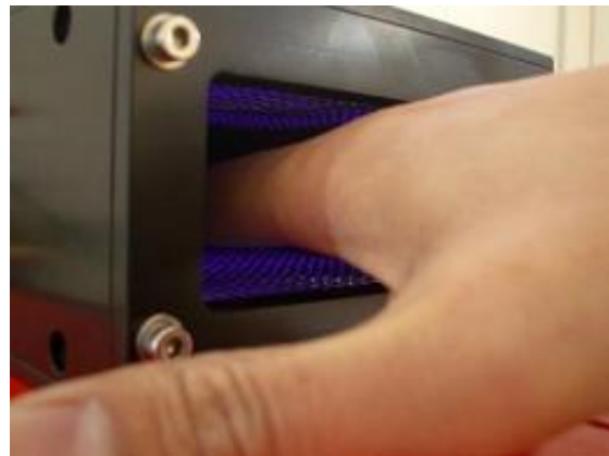
Laboratory prototype plasma device for sanitising hands. Credits: Max-Planck Institute for Extraterrestrial Physics
