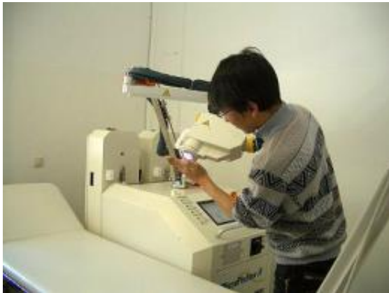
MicroPlaSter beta version of the atmospheric plasma device for chronic wound treatment. Credits: Max-Planck Institute for Extraterrestrial Physics
