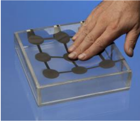
Dielectric elastomer sensors can be customized and applied in a variety of ways. (© Fraunhofer ISC)
