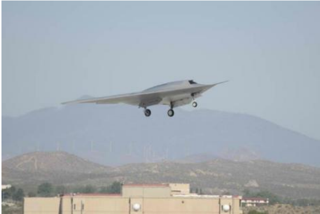
The Boeing Phantom Ray unmanned airborne system (UAS) on its first flight. Credit: Boeing.
