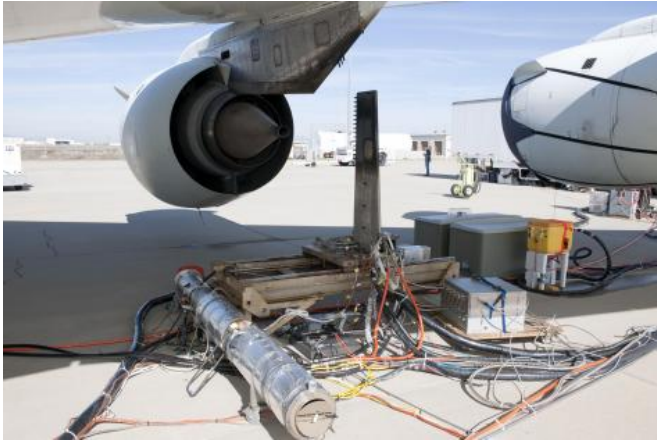
An emissions detection rake device is positioned behind the No.3 engine on NASA's DC-8 flying laboratory during ground tests of an alternative jet fuel made from chicken and beef tallow. Credit: NASA / Tom Tschida
