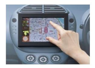
Toshiba Mobile Display has developed a 7.0-inch low-temperature polysilicon (LTPS) thin-film transistor (TFT) liquid crystal display (LCD) for vehicle-mounted and industrial uses that enables multi-touch input on the display screen without the need for additional installation of a touch panel as a demonstration of its new touch panel technology.
