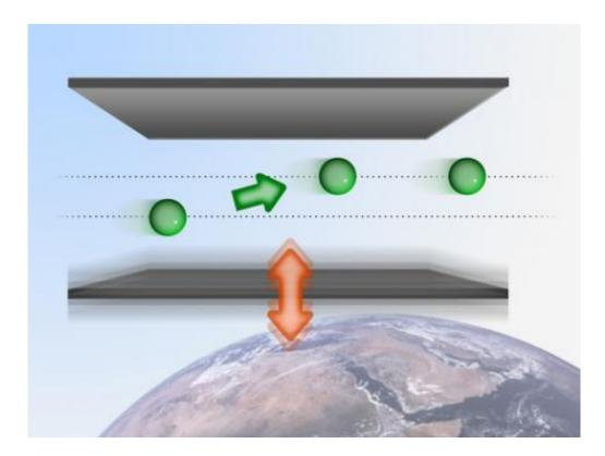
Neutrons between two plates in the earth's gravitational field can occupy different quantum states. A vibrating plate (below) can excite them from one state into the other - which allows extremely accurate energy mearurements.
