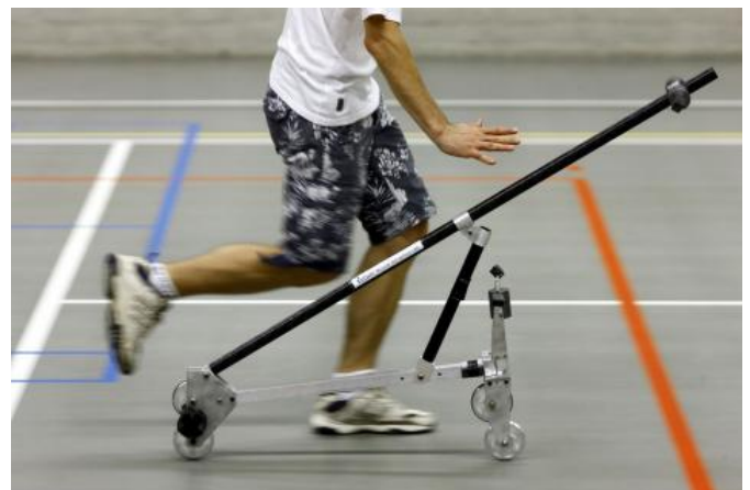
Self-stable experimental TMS bicycle rolling and balancing (photo by Sam Rentmeester/FMAX).
