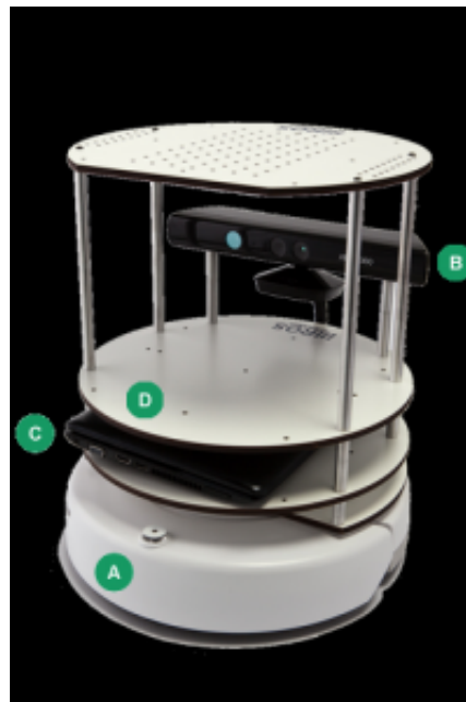
TurtleBot: A Mobile Base and Power Board, B 3D Sensor, C Computing :: ASUS 1215N, D TurtleBot Hardware.
