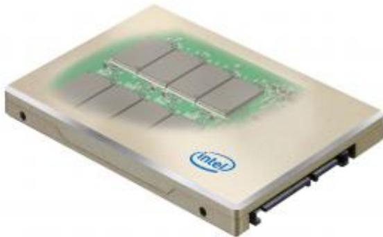
Inside the Intel SSD 510 Series - This photo shows the flash memory inside the Intel SSD 510. Based on 34-nm NAND flash memory, the Intel SSD 510 Series delivers best-in-class sequential performance of up to 500MB/s sequential read speeds and 315 MB/s writes for its high-capacity model. The product is available now and comes in a 250GB capacity priced at \$584 and a 120GB at \$284, for 1,000 unit quantities.
